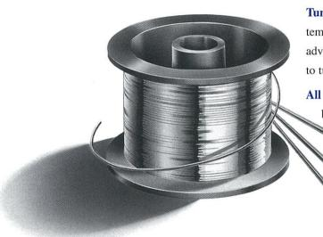
**Tungsten rhenium wire** is used for heating elements in high temperature furnaces, thermocouples and in electronics. Its advantage is its ability to maintain greater ductility compared to tungsten after exposure to extremely high temperatures.
