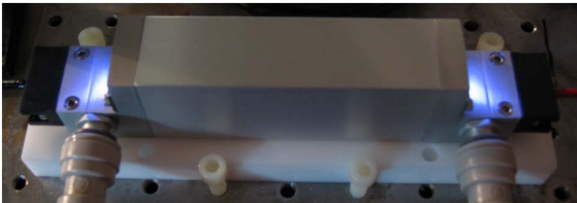
HE7X115F1 Pump Chamber. This pump chamber is specially designed for high energy applications such as material processing or dermatology. Similar in size to our standard pump chambers, the High Energy “HE” line uses our high density composite aloxite diffuse reflector. The HE7X115F1 pump chamber can produce output energies up to 100J.
