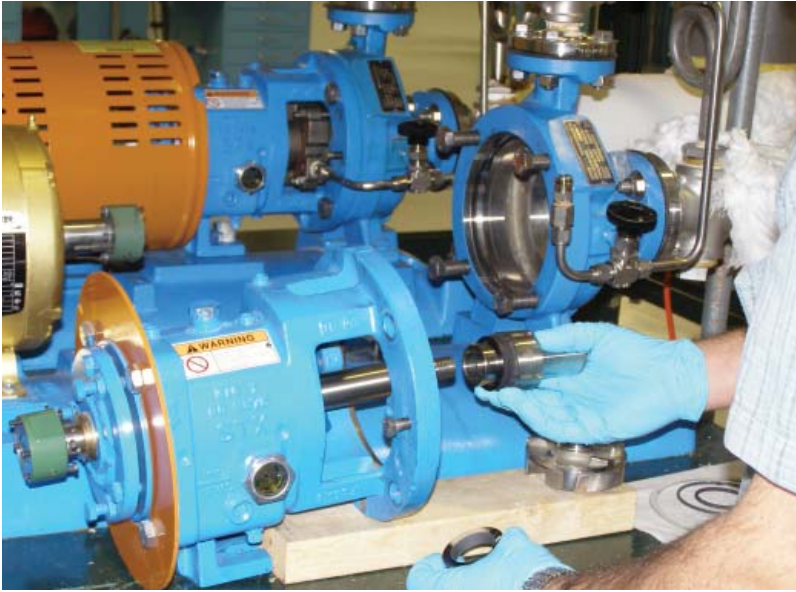
Advanced Diamond Technologies on-site seal testing
