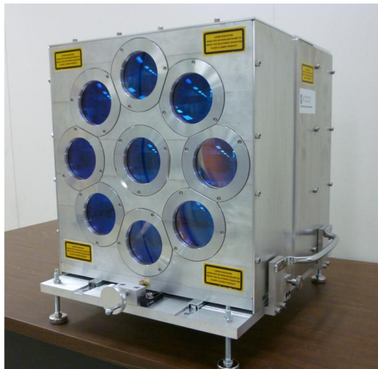
Fig 19. Picture of an illuminator delivering 650W with a beam divergence of 20mR for illumination of a small target at a long distance. The illumination intensity is 50,000 lumens/ sq meter at a distance of 50 meters. The dimensions of the product is 21x17x19 inch.
