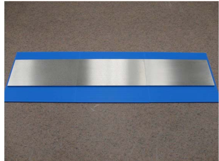
3 CuGa25+ tiles ready for bonding.
