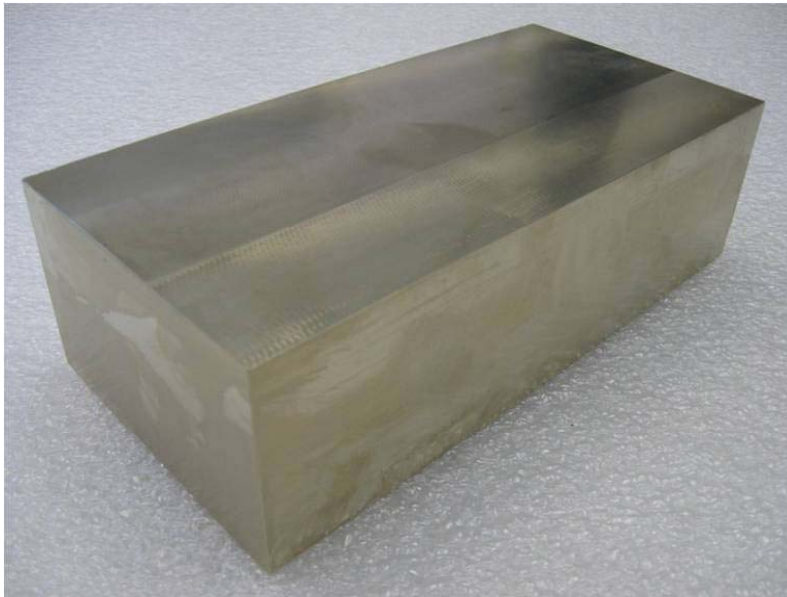
A Typical machined CuGa25 billet
