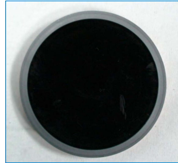
CIGS target after RF sputtering*
