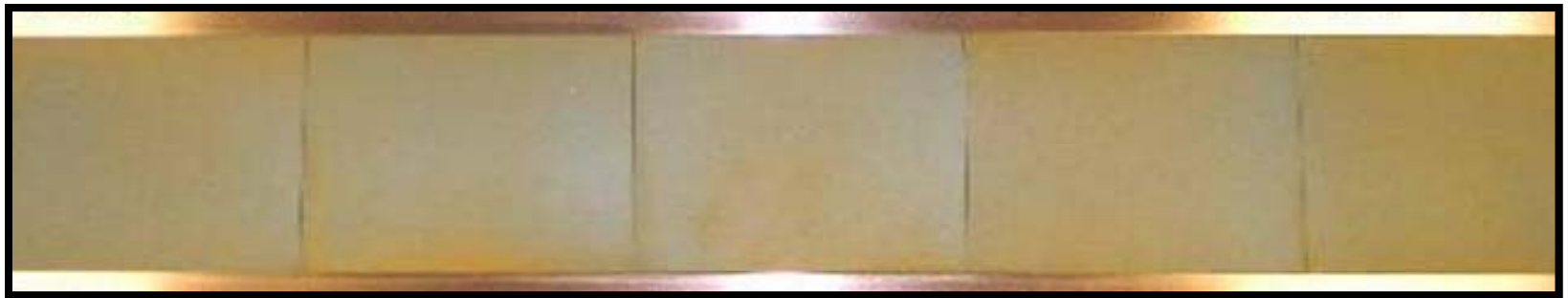
Sequentially bonded CdS tiles (on copper) for a large width sputtering process (March 2011).
