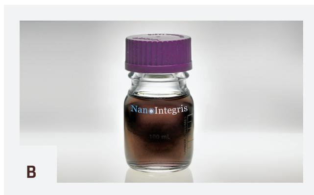
**Figure 1.** 5 mg of (A) MONO (B) and QUATTRO graphene in 100 mL of solution.
